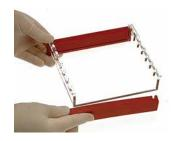
Casting dams allow gels to be rapidly cast externally while the unit is in use for gel running1
